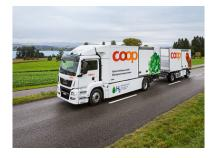
provided the 100kW stack, integrated by SwissHydrogen and ESORO. The electric motor provides a steady 250kW and seven 700bar Luxfer tanks stacked behind the cab give the truck 32kg of usable hydrogen, and a range approaching 400km.
