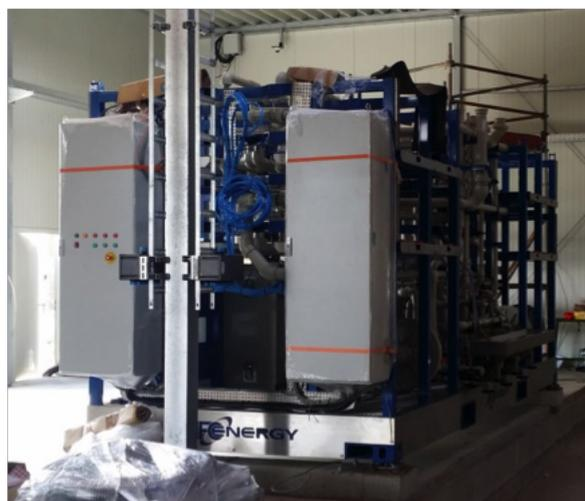
Other technologies remain minor in comparison to the total. Important nevertheless in 2015 is the shipment of alkaline fuel cells by AFC Energy of the UK to its flagship demonstration project in Stade, Germany. This technology appears in the figures for the first time since 2013.
