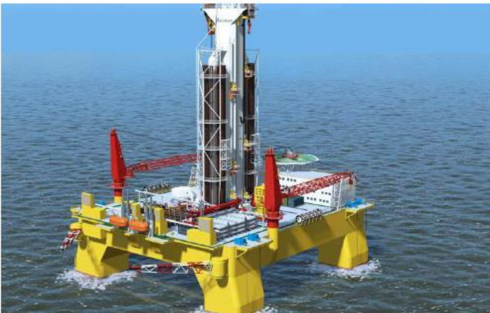
FIGURE 2.2 EXAMPLE OF SEMI-SUBMERSIBLE DRILLING UNIT
