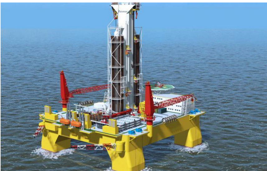
FIGURE 3-2 EXAMPLE OF SEMI-SUBMERSIBLE DRILLING UNIT
