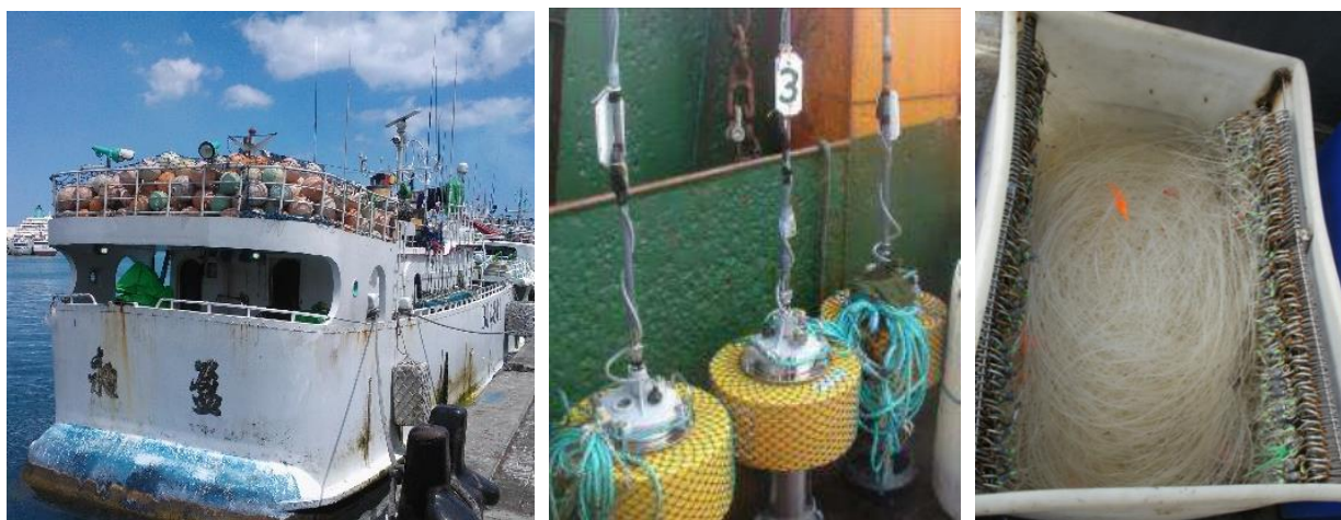
FIGURE 3.4 PHOTOGRAPHS SHOWING MARKER BUOYS (LEFT), RADIO BUOYS (CENTRE) AND MONOFILAMENT BRANCH LINES (RIGHT) (SOURCE: CAPMARINE, 2015).
