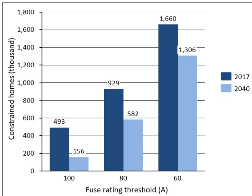
**Figure 7: Number of homes restricted by fuse rating to the installation of air source heat pumps in 2017 and 2040, depending on fuse limits of 100, 80 and 60 A**
