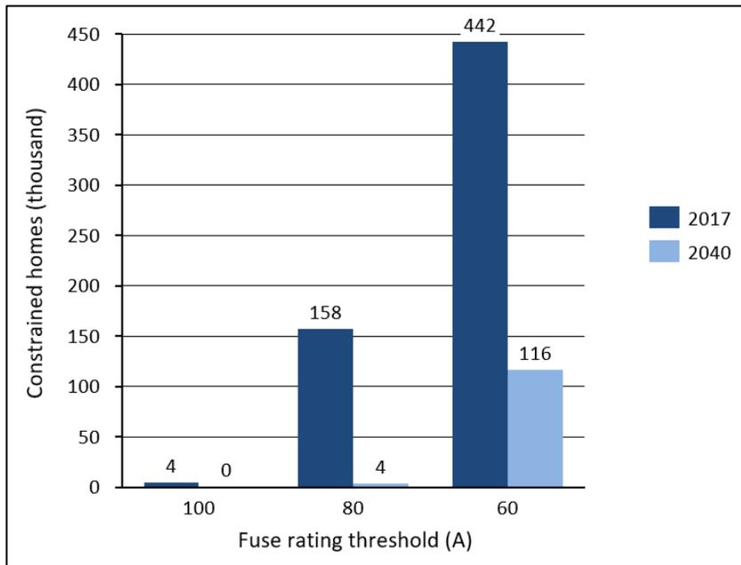
**Figure 6: Number of homes restricted by fuse rating to the installation of direct electric heating in 2017 and 2040, depending on fuse limits of 100, 80 and 60 A**
