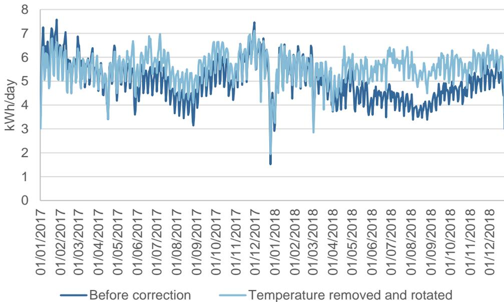
Figure 6-17: Daily demand profile for residential charging before and after influence of temperature is removed and profile is rotated to ensure flat demand trend.
