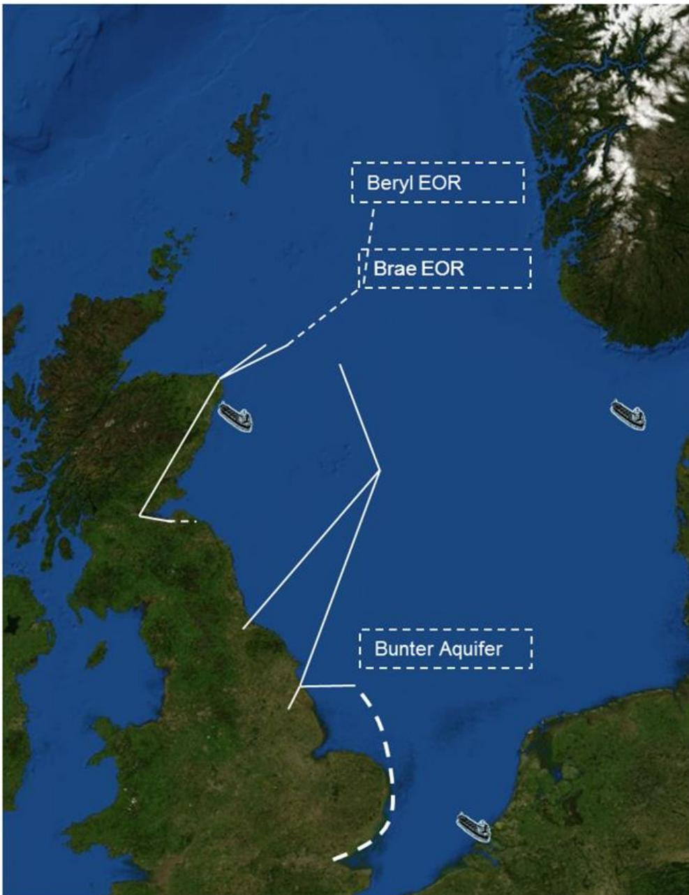
**Figure 30: Infrastructure in 2023-2027. Dashed lines indicate under development. Bold lines indicate operational.**
