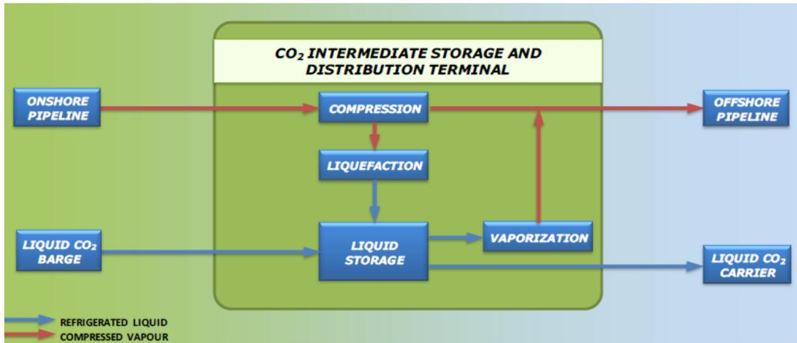
**Figure 39: Port requirements identified for a liquid logistic shipping concept (Vopak, Tebodin, Anthony Veder report for the GCCSI (2013))**
