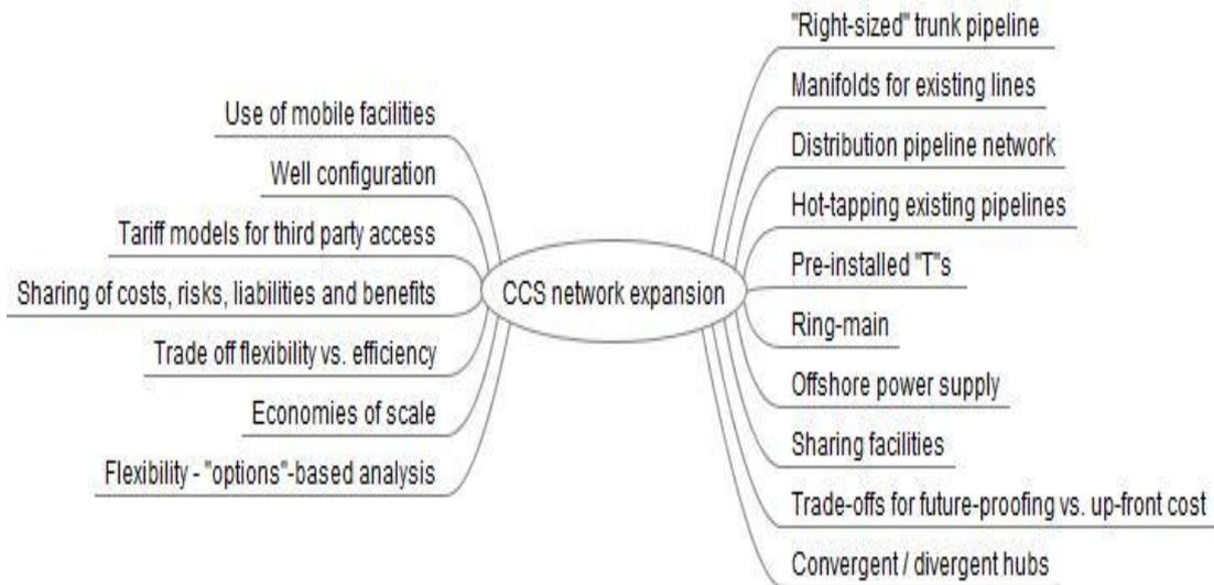
Figure 27: Mechanisms and drivers for CCS network expansion
