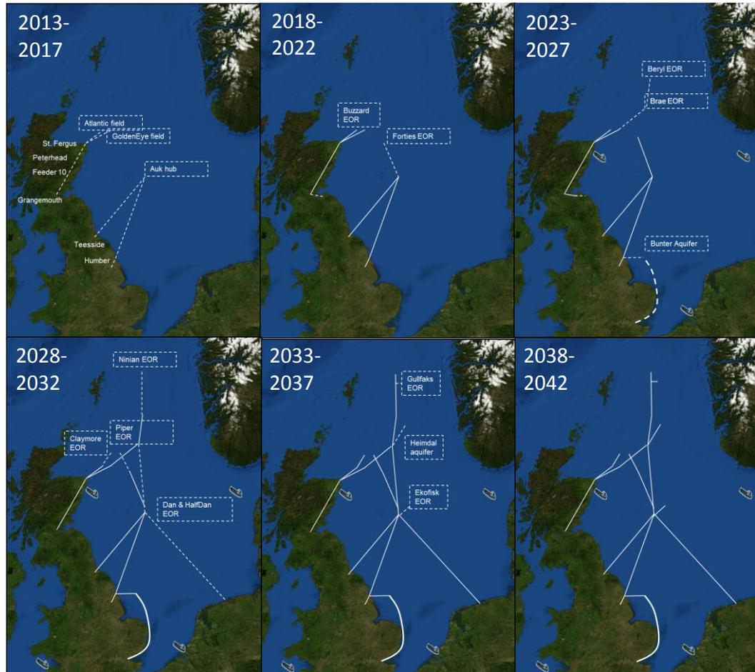
Figure 54: Planned phased infrastructure growth for the Aggressive Scenario indicating investment requirements in six 5-year phases from 2013-2042.
