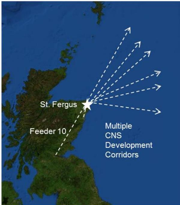
**Figure 2: St. Fergus gas terminal provides access to multiple development pathways, using existing or new pipeline or shipping infrastructure via Peterhead, that can be linked to potential CO<sub>2</sub> storage or CO<sub>2</sub>-EOR locations in the CNS and NNS.**
