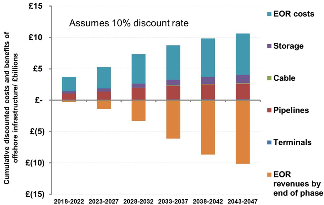
Figure 45: Discounted real offshore costs and revenues for the Aggressive CCS with CO<sub>2</sub>-EOR scenario (assumes DECC central oil price).
