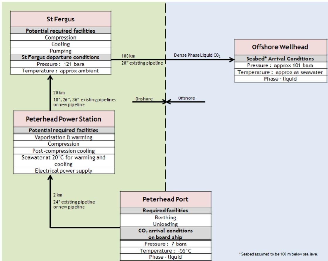
Figure 41: Schematic of CO<sub>2</sub> transport at Peterhead Port considered by Petrofac
