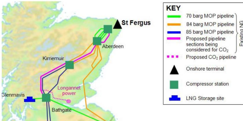
**Figure 18: The sections of the Feeder 10 pipeline that were examined by National Grid for re-use with CO<sub>2</sub> (in pink) (Image copyright National Grid, reproduced from DECC Longannet-Goldeneye CCS FEED study).**
