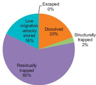
**Figure 11: A mixture of trapping mechanisms can operate - the figure shows the predicted role of different mechanisms in a typical large dipping aquifer such as the Forties aquifer in the CNS 1,000 years following CO<sub>2</sub> injection. (Goater et al. 2013)**
