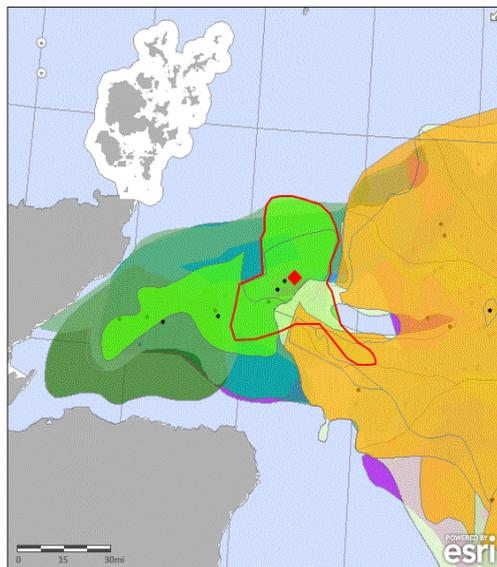
**Figure 12: Captain sandstone saline aquifer has a large area, irregular shape, overlaps other stores. Colours show other storage sites in the different stratigraphic layers, red dot shows the centroid of the polygon).**
