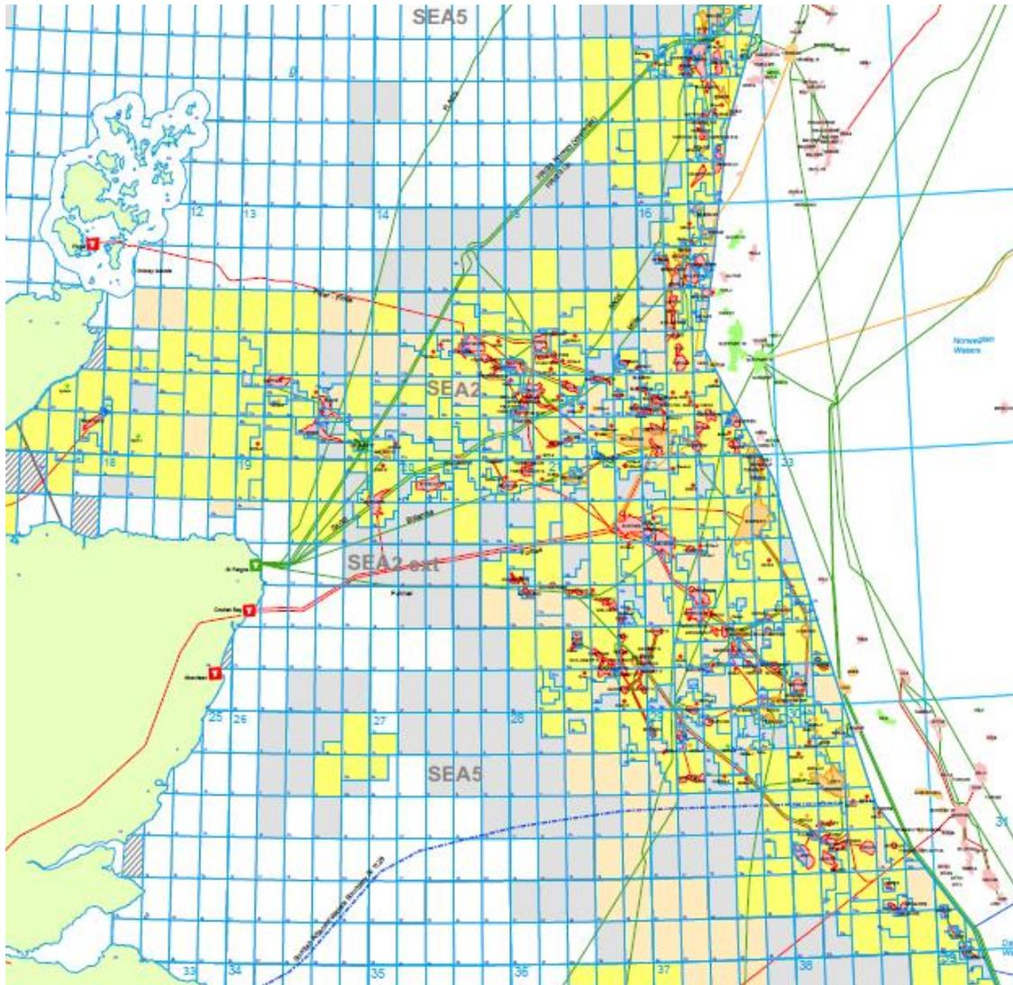
Figure 26: Illustration of existing pipeline infrastructure in the Scottish territorial waters of the central North Sea. Green lines = gas pipelines; Red lines = oil pipelines. Yellow squares – licensed oil and gas blocks.
