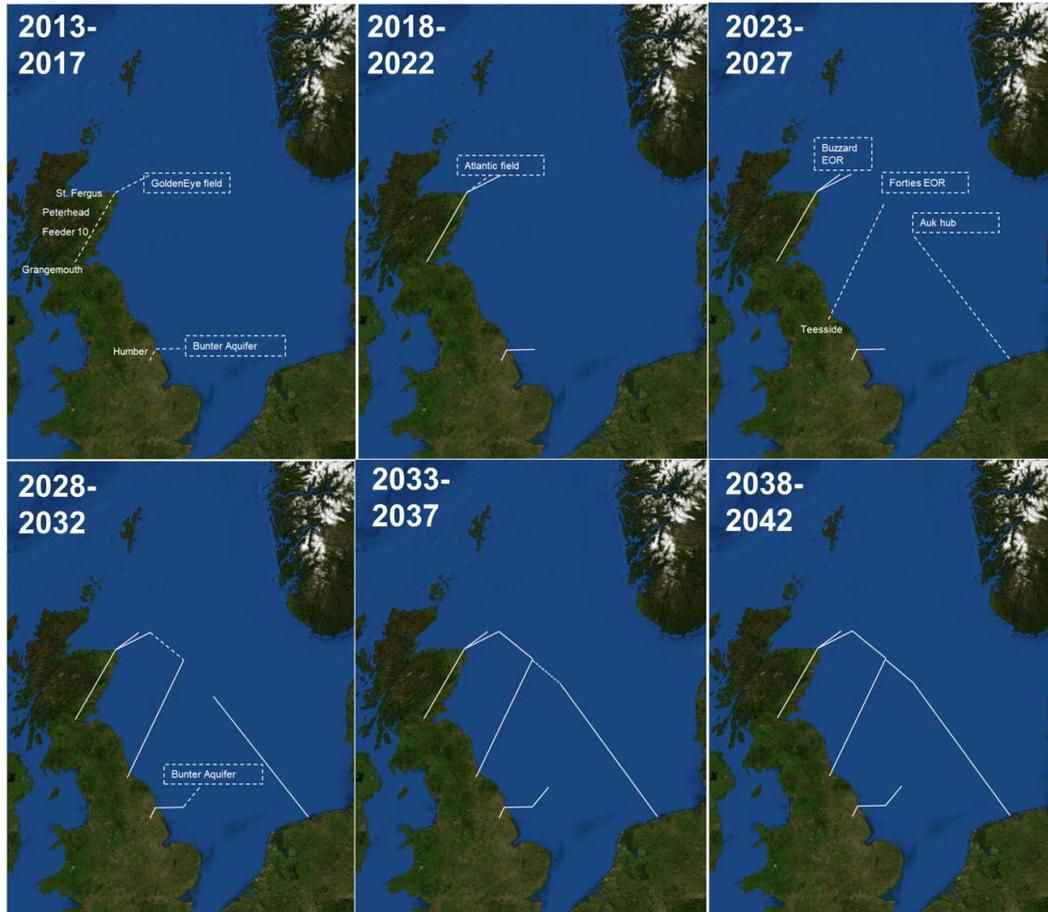
Figure 36: Cautious CCS with EOR network development. Dashed lines indicate construction/development, bold lines indicate operational pipeline infrastructure.
