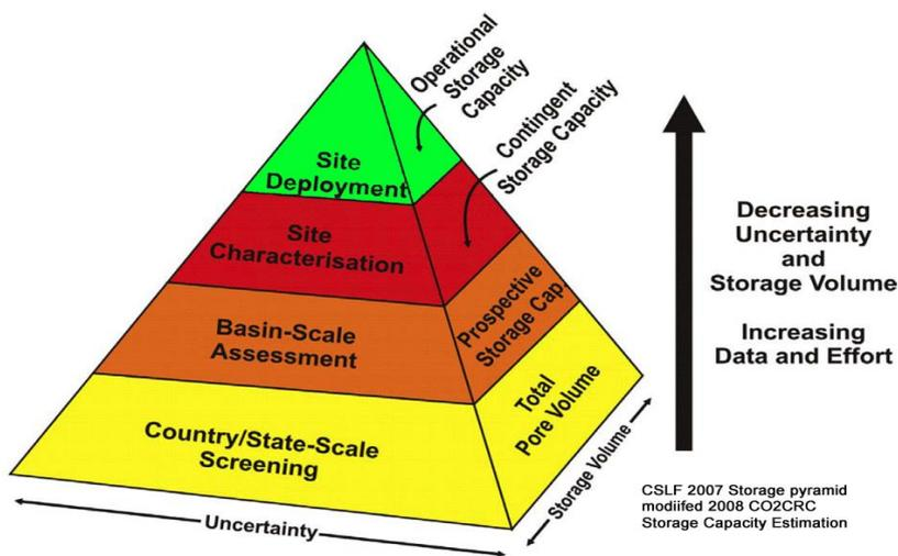
**Figure 10: Resource pyramid illustrating developing assessment of geological CO<sub>2</sub> storage capacity**
