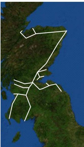
**Figure 20: Hypothetical "all Scotland" onshore pipeline network connecting 28 planned or existing CO<sub>2</sub> point source emitters in Scotland.**
