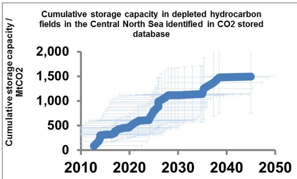
Figure 13: Cumulative capacity in depleted hydrocarbon fields in the central North Sea over time, assuming all fields become available on cessation of production.
