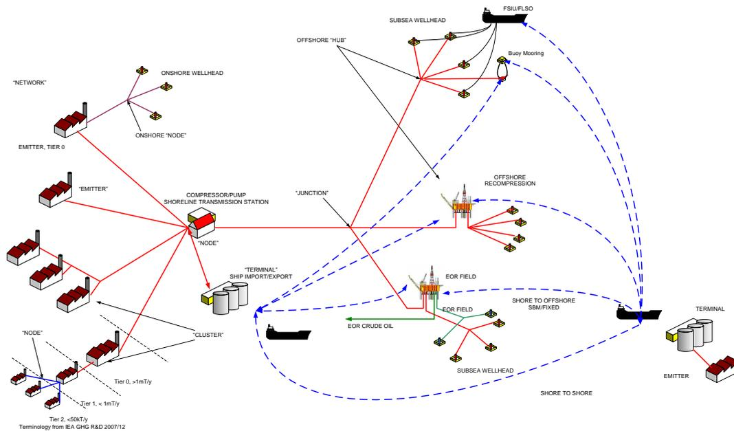
**Figure 38: Diversity of potential CCS network configurations involving CO<sub>2</sub> shipping**
