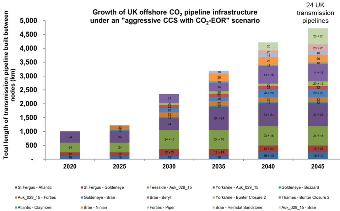
Figure 34: Growth in CO<sub>2</sub> pipeline infrastructure for the Aggressive CCS with CO<sub>2</sub>-EOR scenario. Each colour reflects different network nodes. Figures inside the bars reflect the diameter of pipelines (in inches).
