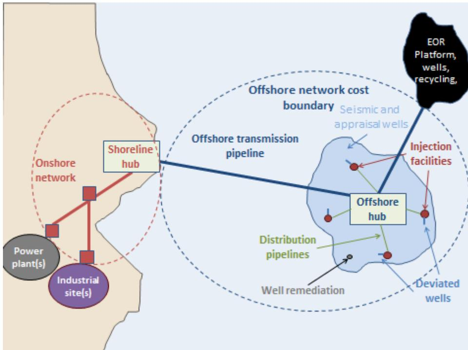
Figure 44: Scope of contributing models for infrastructure cost analysis used in this study.
