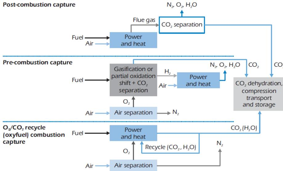
**Figure 2 Dominant approaches to CO<sub>2</sub> capture (Image reproduced from IEA (2008) CO<sub>2</sub> capture and storage – a key abatement option).**
