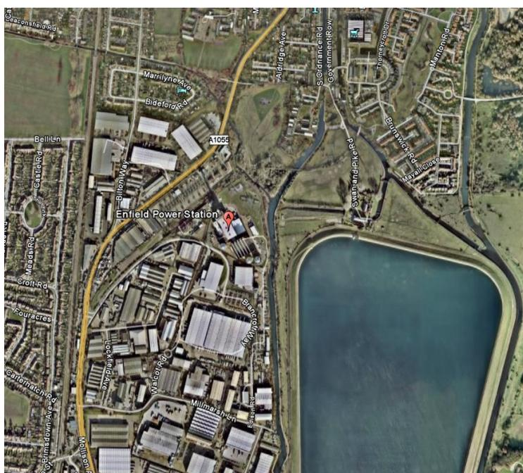
Here the site is almost fully bound. Access to the South, West and North is via industrial or residential areas severely limiting pipeline access. To the East is a reservoir. There is a very narrow route in the North-East.
