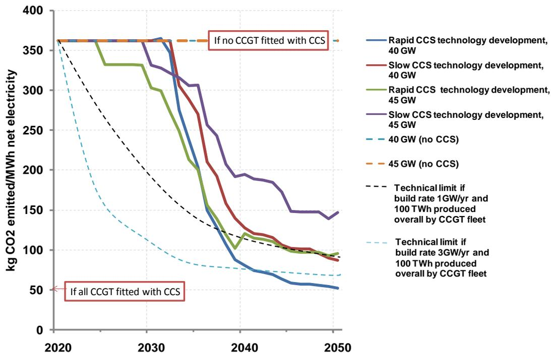
Figure 37 CO<sub>2</sub> intensity of energy generated from the gas fleet through time, under various scenarios. The technical limit for technology readiness in 2020 is also shown.
