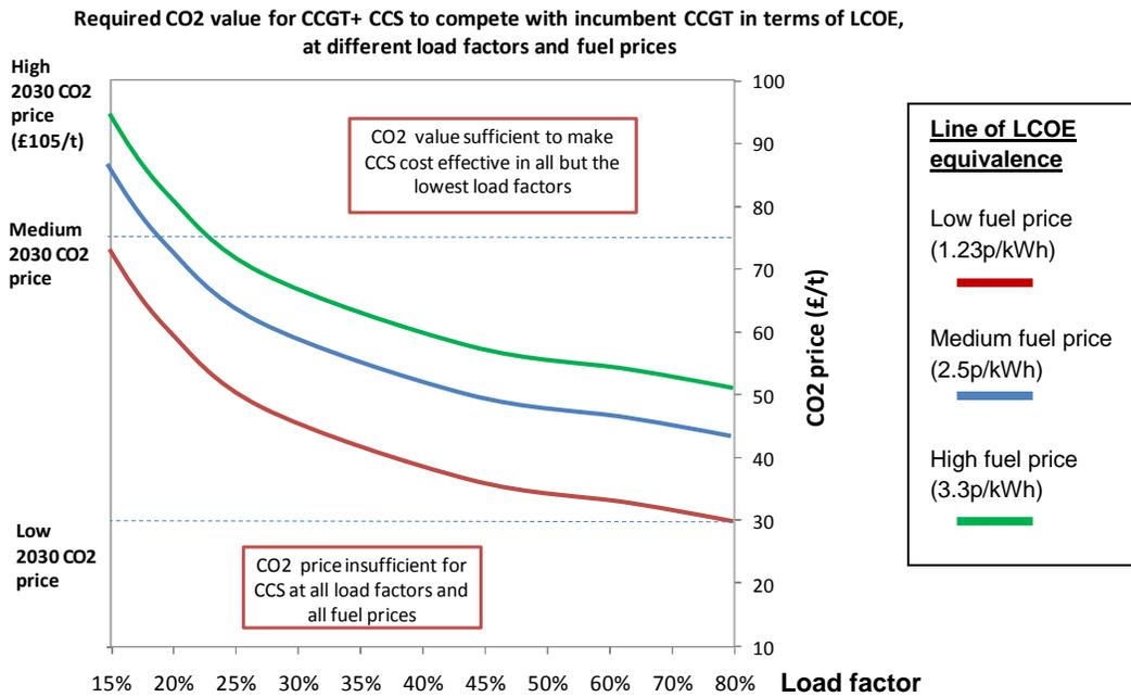
**Figure 33** The impact of fossil fuel price on the CO<sub>2</sub> value required for the LCOE of a refurbished plant with CCS to equal that of a plant without, for a given load factor
