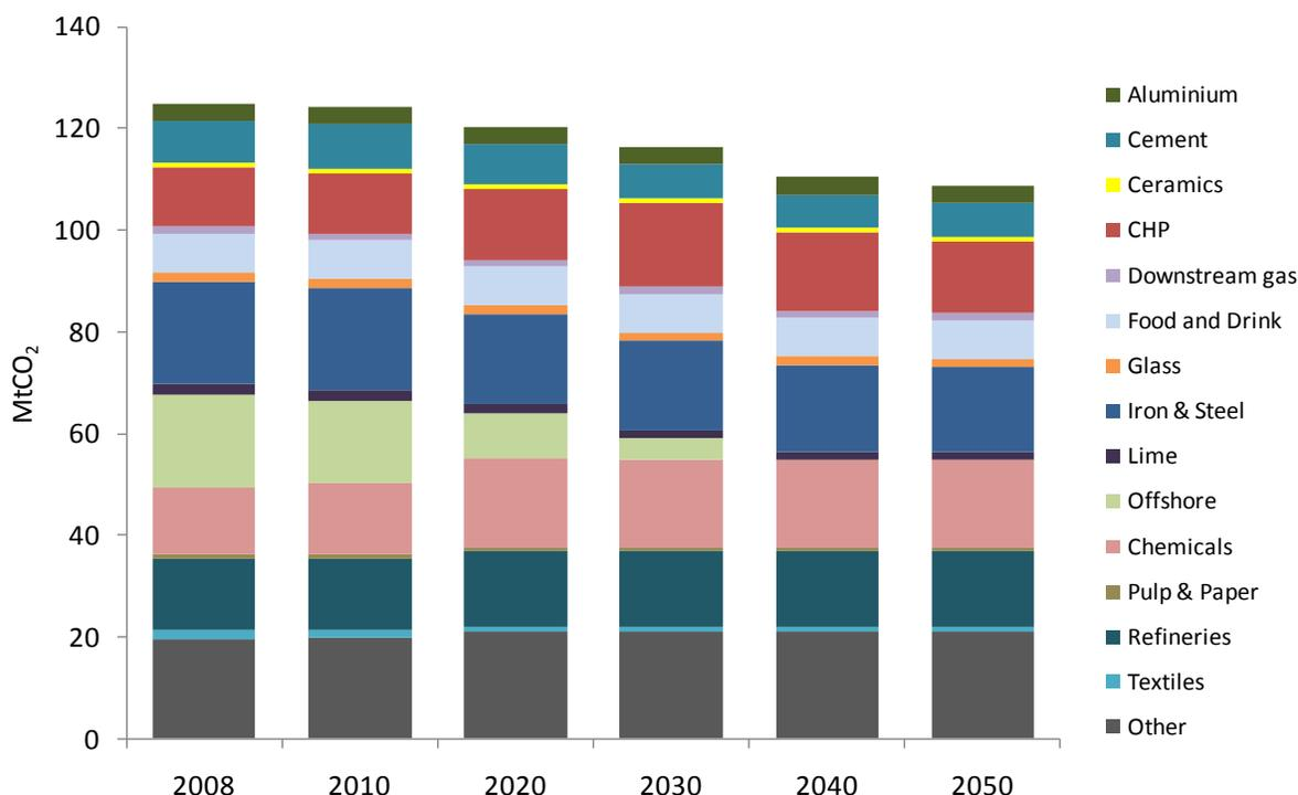
The base case forecast projects CO<sub>2</sub> emissions from industry to fall from 125 MtCO<sub>2</sub> in 2008 to around 120 MtCO<sub>2</sub> in 2020 and 109 MtCO<sub>2</sub> in 2050, representing a decline of 13% over the period 2008-2050. The forecast compares against the UK Low Carbon Transition Plan ‘central’ projection of industry emissions including refining falling to 120 MtCO<sub>2</sub> in 2020<sup>12</sup>.
