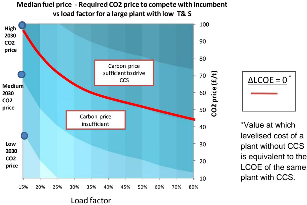
The penetration of CCS through the gas fleet is clearly dependent on CO<sub>2</sub> price trajectory and load factors, but also to technology readiness. In fact, technology readiness may be the limiting step in adoption of capture in the 2020-2030 period. Following this, capture could be taken up by the fleet very quickly, under a variety of CO<sub>2</sub> price trajectories.
