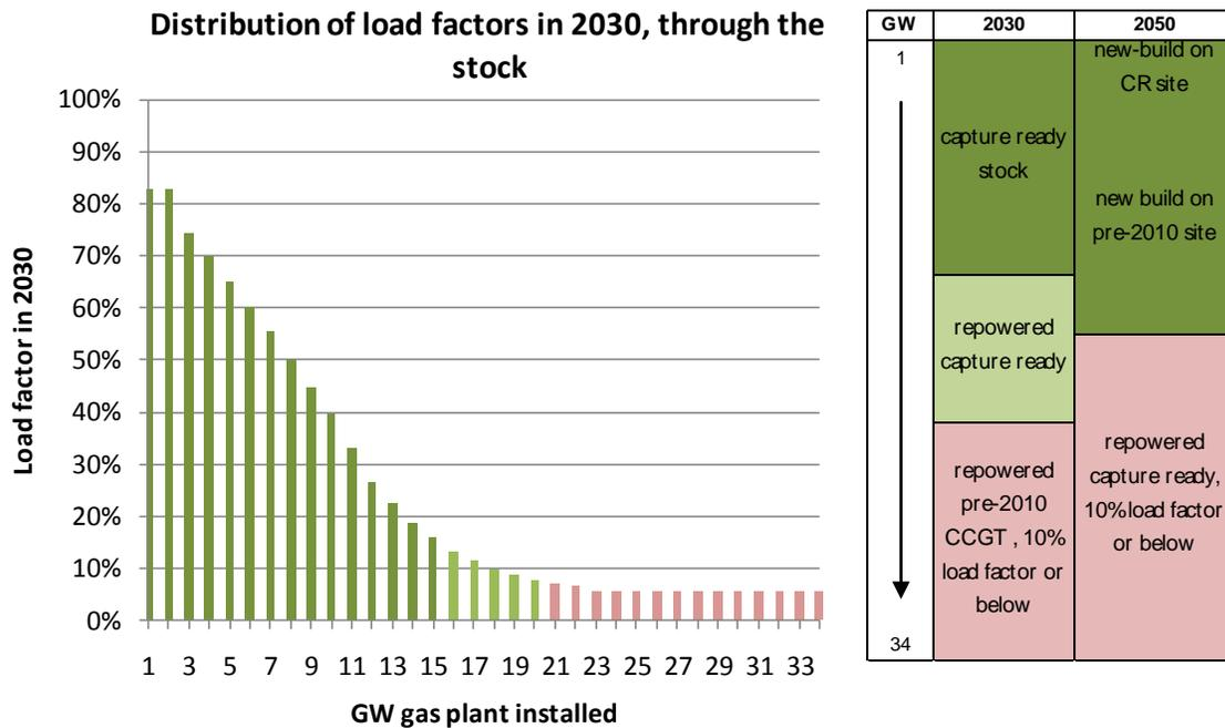
**Figure 34 Load factor distribution amongst the 2030 and 2050 stock**
