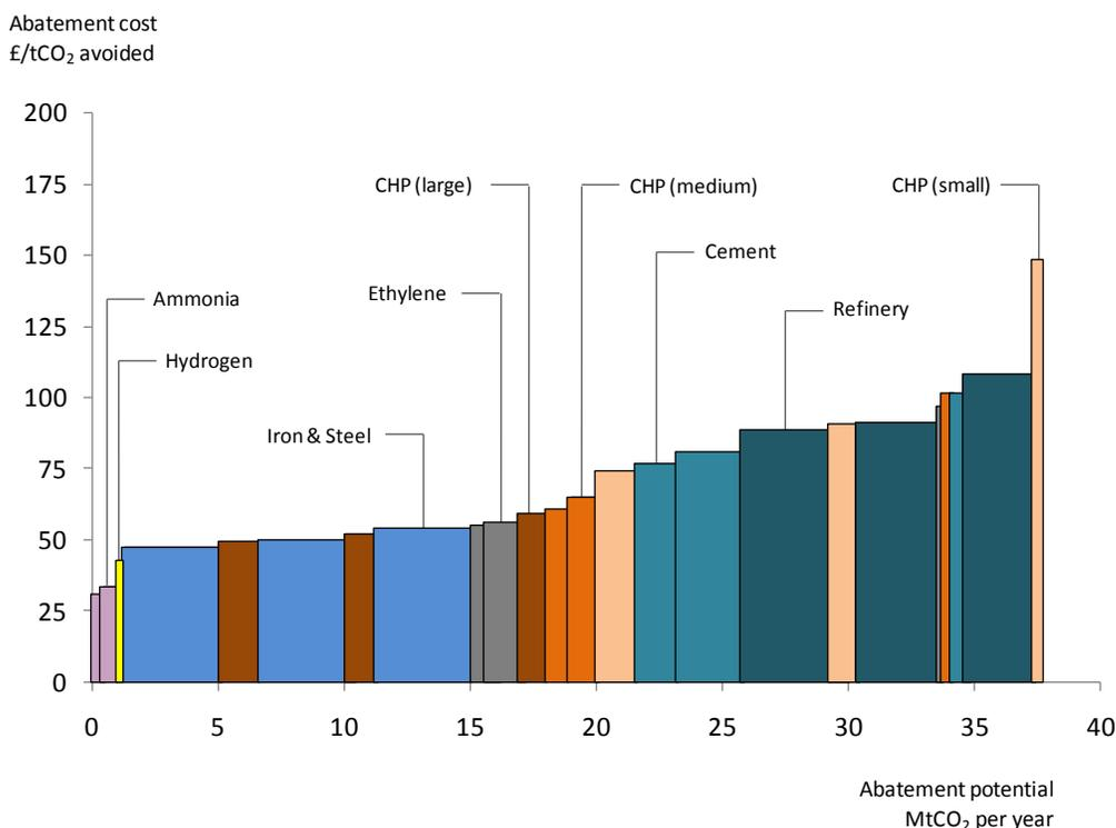
The lowest cost options for industry CCS consist of, in order of abatement potential: iron and steel blast furnaces, larger CHP facilities, and high purity CO<sub>2</sub> streams such as those produced from ammonia and hydrogen production plants. These can deliver the first 15Mt of CO<sub>2</sub> abatement below or around £50/tCO<sub>2</sub> abated.
