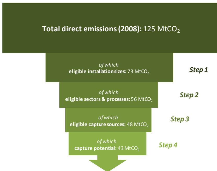
The sites identified as potential capture sites (i.e. Step 2) are shown in *Table 2*.Based on the above methodology, a forecast of technical capture potential (excluding capture from additional capture-related emissions) was calculated, as shown in *Figure 9*. Unless specific plant details were identified demonstrating 2008 emissions data to be unrepresentative, future
