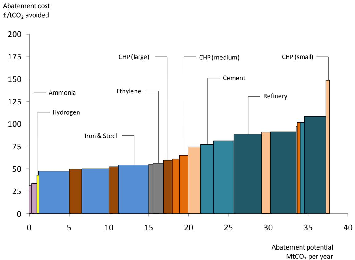
It can be seen that around one third of the abatement potential is estimated to be achievable at around £50 per tCO<sub>2</sub> or less and includes capture from high-CO<sub>2</sub> stream ammonia and hydrogen plants, the three integrated iron and steel works and the majority of large-scale industrial gas-fired CHP capacity). A further third of the potential is available for around £80 per tCO<sub>2</sub> or less (capture from ethylene plants and most medium-scale CHP units and cement
