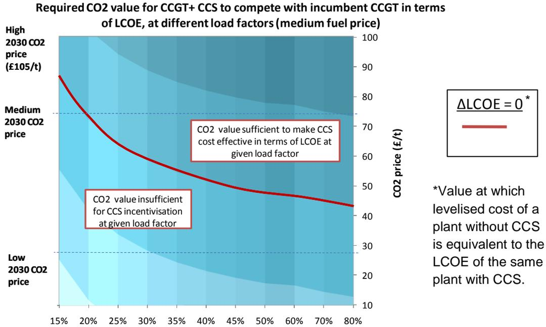
**Figure 32** CO<sub>2</sub> value required for the LCOE of a refurbished plant with CCS to equal that of a plant without, for a given load factor.
