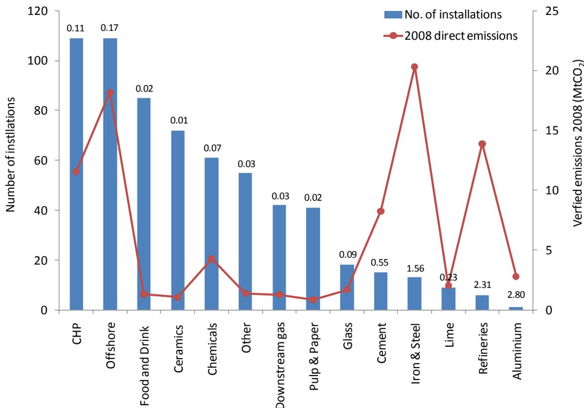
Note: figures shown above columns indicate average sector direct CO<sub>2</sub> emissions per installation in MtCO<sub>2</sub>/yr
