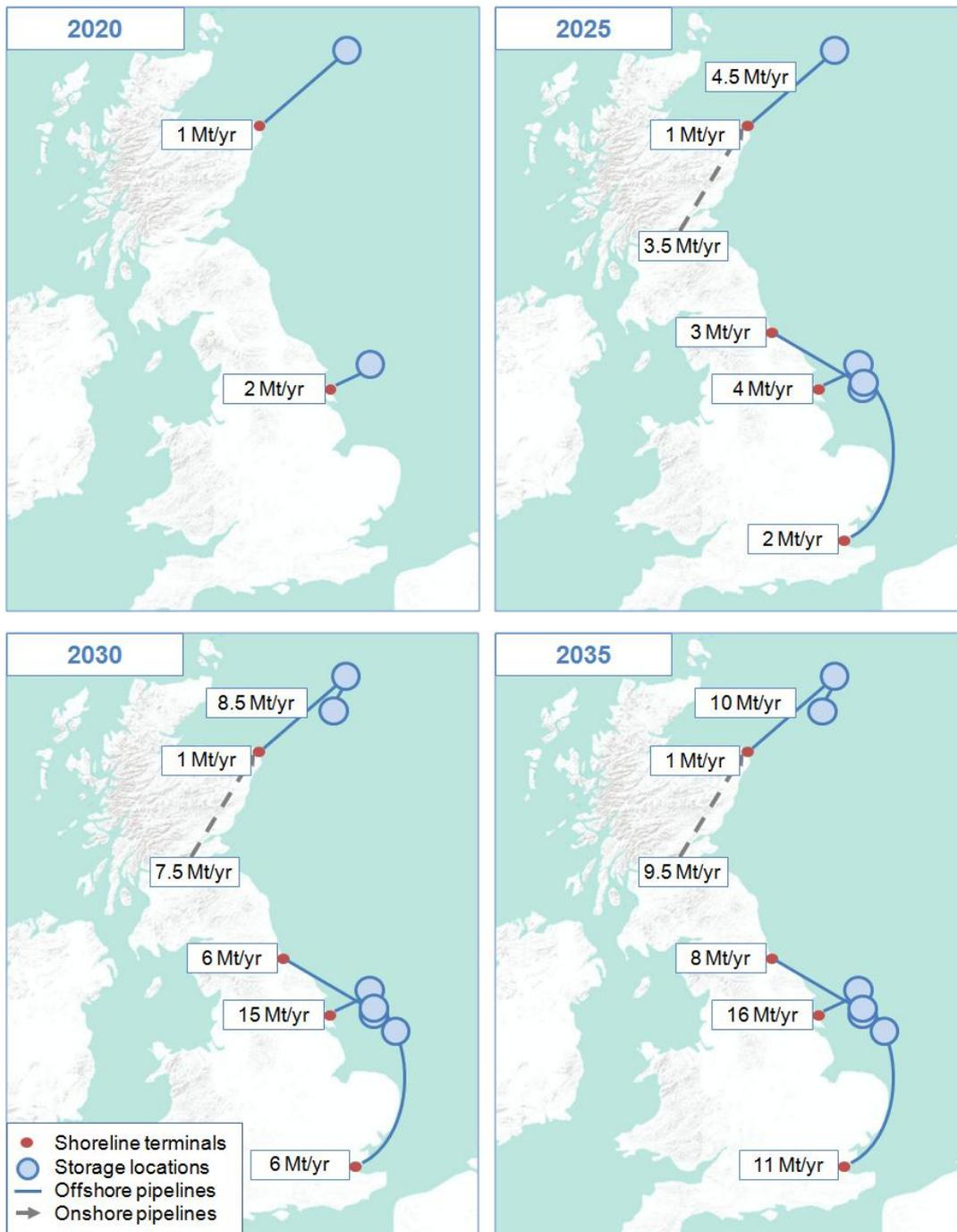
Figure 5: Snapshot maps of the CCS networks in the delayed electrification scenario<sup>10</sup>
