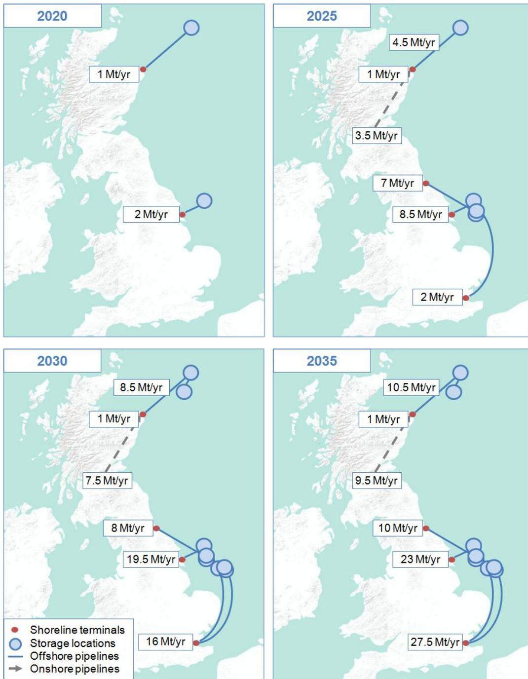
Figure 3 Snapshot maps of the CCS networks in the core decarbonisation scenario.<sup>8</sup>
