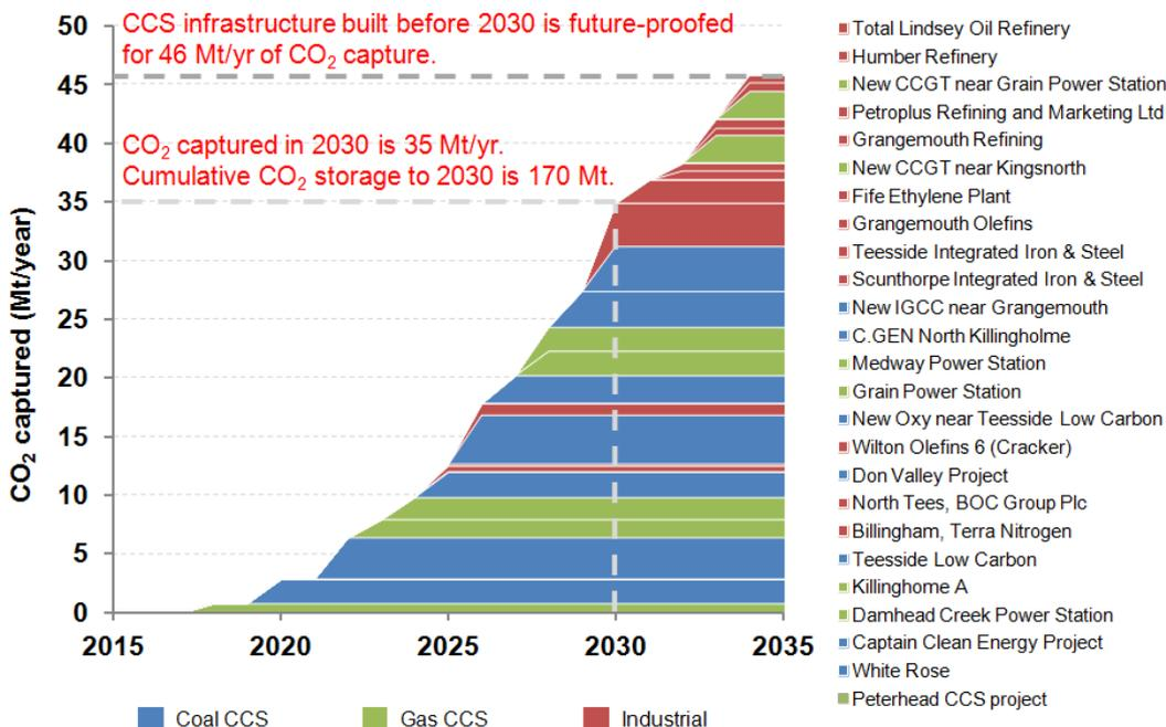
Figure 4: CO<sub>2</sub> capture in the delayed electrification scenario<sup>9</sup>
