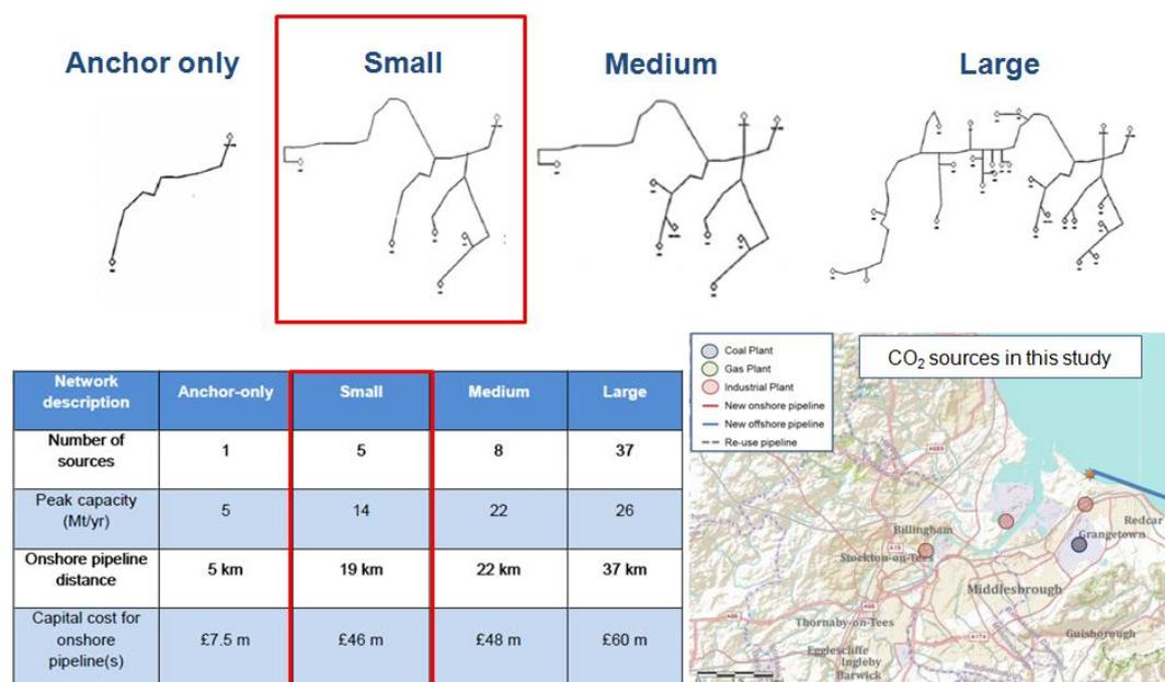
Figure 17: Onshore pipeline network in Teesside<sup>28</sup>
