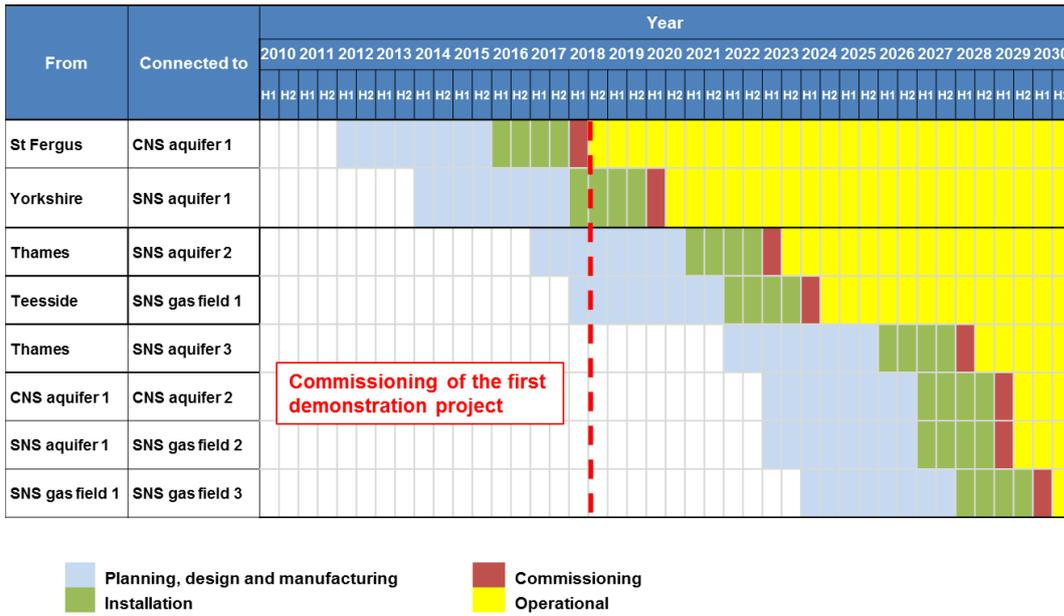
Figure 21: Offshore pipeline development in the core decarbonisation scenario
